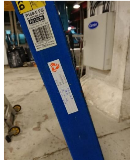
Registration label for equipment brought by subcontractors
