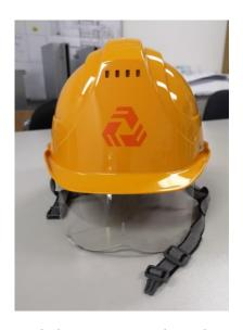
A helmet equipped with a retractable goggle
